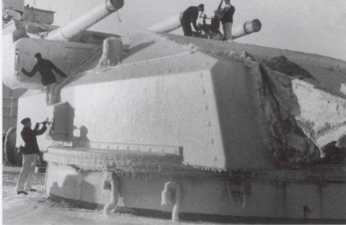
Sailors chip rime ice from hatches on GNEISENAU's A main turret during Operation BERLIN. This thin ice coating did not affect the ship's stability, but it was necessary to remove it from hatches, including the doors that covered the main battery turret rangefinder optics. A 20mm Flak 38 cannon is mounted atop this turret. (Bundesarchiv)
