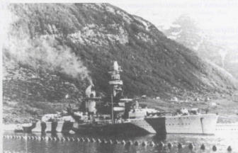
LÜTZOW was based at Narvik, Norway in the early Summer of 1942. She was painted in a splinter camouflage of Dark Gray on a Light Gray background. The idea behind this camouflage was that, at a distance, the two shades blended into a Medium Gray that faded into the horizon. Close up, the splinters were difficult for split prism rangefinders to focus on. LÜTZOW was retrofitted with the elongated 'clipper' bow similar to that on ADMIRAL SCHEER. (NHC)
