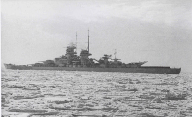
GNEISENAU's crew is mustered aft while she is locked in ice prior to Operation NORDMARK in February of 1940. An Arado Ar 196 floatplane is spotted on her amidships catapult, but no aircraft is located on GNEISENAU's aft turret catapult. The latter catapult was not employed early in World War Two and was removed from the ship by 1942. (Bundesarchiv)
