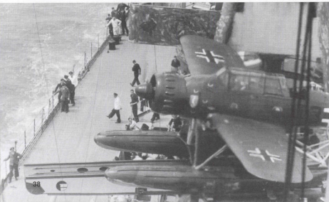
This same Ar 196A-4 (T3+EK) is launched from ADMIRAL SCHEER's catapult. This aircraft was deployed to seek targets in the calm South Atlantic. Its flaps were fully lowered for launch. The launch cradle ran to the end of the catapult. The Ar 196 was a faster aircraft than the He 60C and proved well suited for shipboard operations. (NHC)
