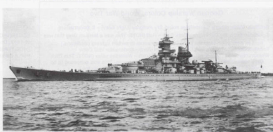
The new GNEISENAU is depicted on a propaganda postcard. The ship is pictured above the lyrics of a German patriotic song, "Denn wir fahren gegen England!" ("Then we sail against England!"). During late 1938, GNEISENAU was fitted with a modified 'Atlantic' clipper bow and a tall funnel cap. Unlike her sister SCHARNHORST, GNEISENAU's main mast remained immediately aft of the funnel.
